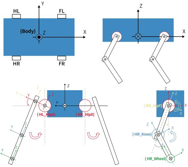
\*The arc-shaped arrow indicates the positive direction of rotation for the joint coordinate system with the same color.
