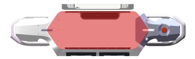
The pass through for official cables is located on the back of the robot. When designing the backload, it is necessary to reserve at least 10mm from the top of the mounting rail as space for wiring.
